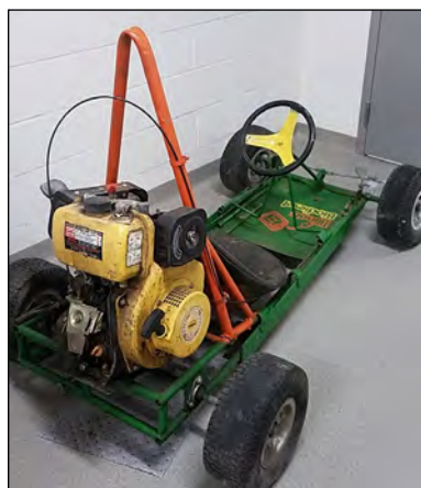
IBI uses this engine to test the biodiesel it manufactures.
