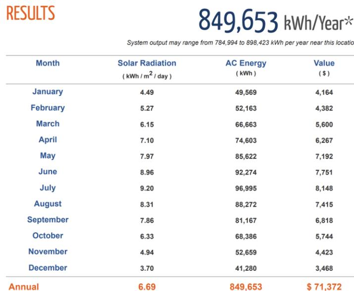
Figure 15: Two-Axis Thin Film Tracking Results
